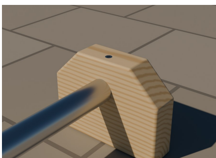
An end block: the rail screwed through from the top
